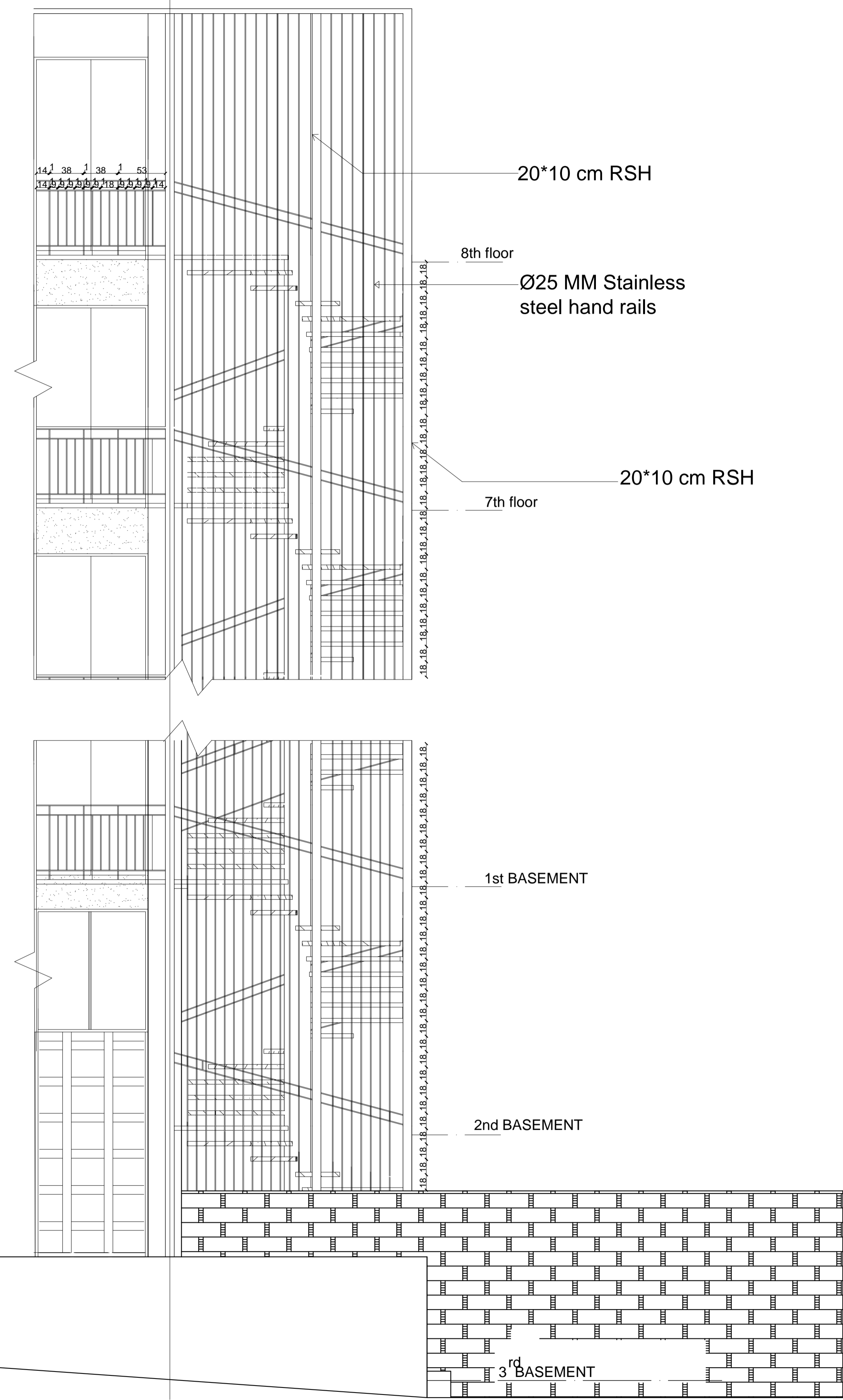
stair Elevation SC 1/20
